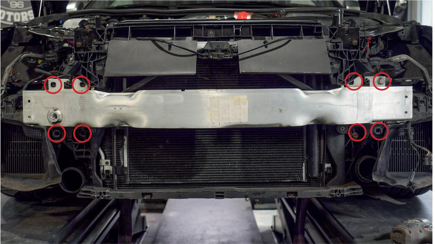
3. Install the supplied support plates at the positions of the baffle bracket using a 16mm nut and the previously removed screws.
